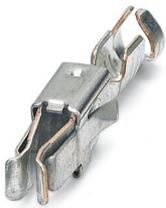
Module female contact, is inserted into the MSTBC connector shell after the conductor has been crimped, for conductors from 1.5 - 2.5 mm<sup>2</sup>, ribbon contact
