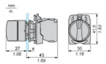
$\boldsymbol{e}\text{:}$  clamping thickness: 1 to 6 mm / 0.04 to 0.24 in.
