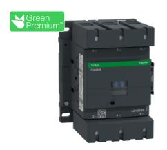
Contactor, TeSys Deca, 3P(3NO), AC-3/AC-3e, <=440V, 150A, 415V AC 50/60Hz coil, screw clamp terminals
