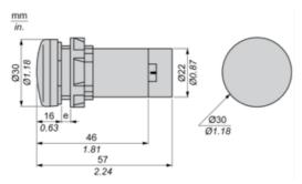
e Support panel thickness: 1 to 6 mm/0.4 to 0.24 in. (metal), 2 to 6 mm/0.8 to 0.24 in. (plastic).
